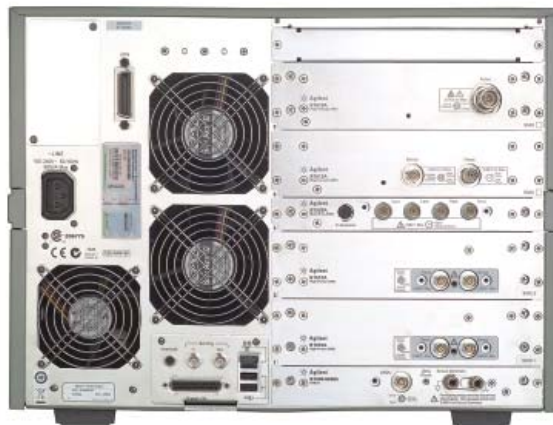
The B1505A 10-slot mainframe supports a variety of modules for high power test.
